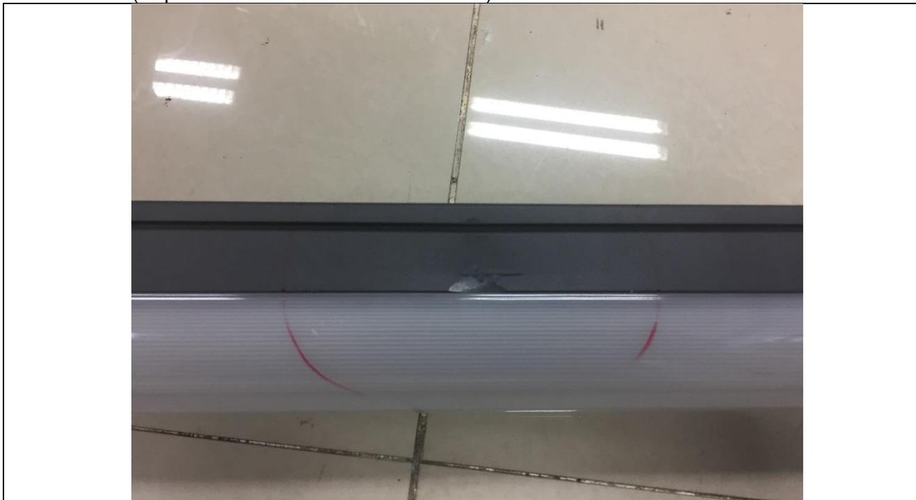
Details of: Metal end cover enclosure view after impacting test
